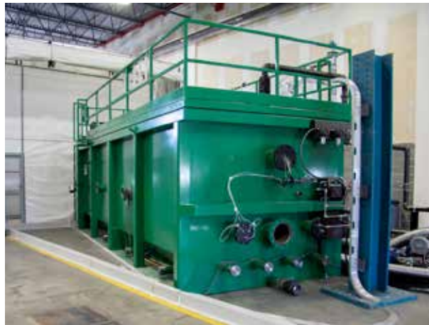
The Enbridge ELDER apparatus, which identifies the best external leak detection technologies on the market, will help to improve pipeline safety across the industry.
